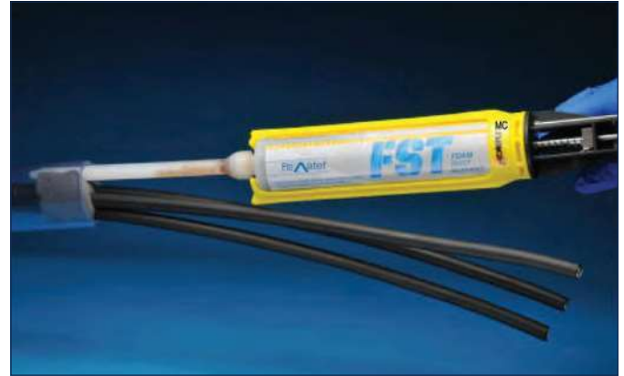
The FST™ Sealant comes in a caulking style (one plunger) tube. Package allows multiple seals. Mixing is done in the nozzle as the sealant is injected.
